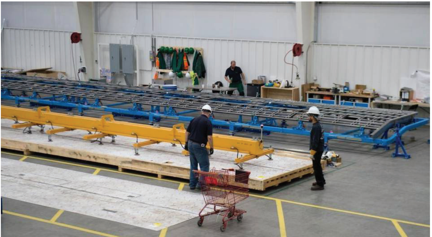
Employees at the Siemens factory in south Sacramento lay out the side panel of a train on Thursday, Oct. 15, 2015. Hector Amezcua hamezcua@sacbee.com
